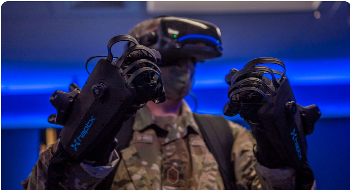
Chief Master Sgt. Mark Umfleet, 317th Airlift Wing command chief tests HaptX Gloves Development Kit 2 at Dyess Air Force Base. Introducing virtual reality gloves into a training environment allows students to feel each action as it is performed.
